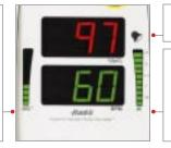
The Alarm Status Indicator flashes when an alarm condition is present.
